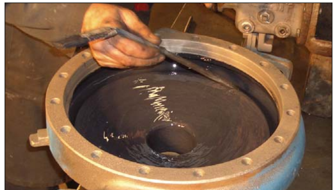
Coating a pump volute with Loctite® Nordbak® Brushable Ceramic
